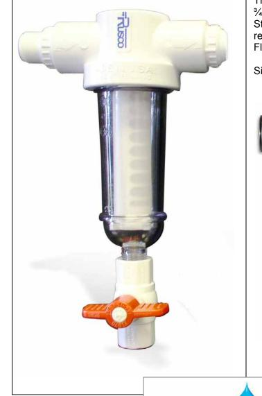
The Self-Cleaning Sediment Filter is available in <sup>3</sup>/<sub>4</sub>" or 2" in/out PVC construction. Stainless steel filter screens, cleanable and reusable. Flow rates up to 50 GPM.
